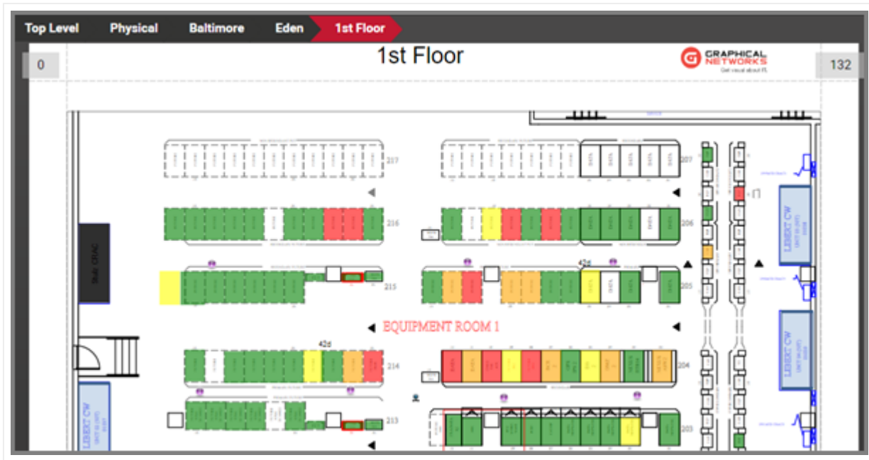
Floor plan view with trays modeled as links and other connections filtered out in layers
